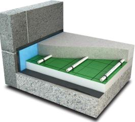
Insulation panels have been developed specifically for use with concrete screeded floors and for liquid flow screeds. Comprising a rigid polyurethane material it has a High Density Polyethylene Woven Film bonded to its upper surface. This protects the insulation from the screed and allows the under floor heating pipe work to be fixed to the panel using specially designed "U" shaped plastic staples.
